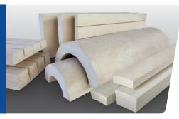
Thermo-1200®\* is a water-resistant, molded, high-temperature, abuse-resistant pipe and block insulation composed of hydrous calcium silicate. Recommended for use in the industrial processing and power generation industries. Integral to Thermo-1200 is XOX Corrosion Inhibitor®, a distinctive formula and process that actively inhibits corrosion to outside surfaces of pipe and equipment.
