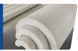
Sproule WR-1200 is a preformed, high-temperature, non-wicking, hydrophobic pipe and block insulation composed of expanded perlite that is uniformly reinforced with a high-strength fiber. Integral to Sproule-1200 is XOX Corrosion Inhibitor®, a distinctive formula and process that actively inhibits corrosion to outside surfaces of pipe and equipment.
