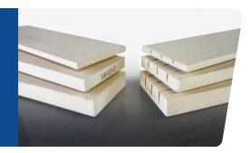
Super Caltemp® Gold 1700 block is an inorganic, noncombustible, high-temperature insulation that is composed primarily of hydrous calcium silicate. The insulation is tailored for systems operating up to 1700°F (927°C). Super Caltemp Gold 1700 meets or exceeds the physical and thermal property requirements of ASTM C533, Type II.
