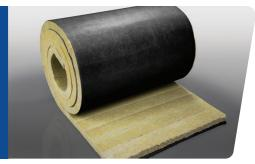
MinWool-1200® Lamella Tank Wrap is a water-repellent, lightweight, strong, flexible mineral wool wrap insulation with perpendicular oriented fibers. This insulation is produced to fit large diameter pipes, ducts, tanks and equipment, operating at temperatures from below ambient up to 1000°F continuous maximum service temperature.
