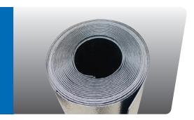
JM's 1 lb Muffl-Jac® sound barrier jacketing is a special high density, composite film laminated to 0.020" aluminum using a viscoelastic film adhesive. It simultaneously absorbs, dampens, blocks and isolates sound, and reduces noise levels radiated by piping and equipment.
