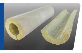
MinWool-1200® Preformed (PF) pipe insulation is a water-repellent, factory v-grooved mineral wool board that is formed to specific pipe sizes. It is provided in half-cylinder sections with a variety of facing options. PF Pipe insulation is a factory "V-grooved" mineral wool board that is formed to specific pipe sizes and provided in half cylinder sections with a variety of facing options.
