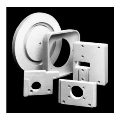
arinite I structural insulation is a non-asbestos incombustible material manufactured in 4' x 8' panel form. These boards are designed to combine structural strength and high thermal insulating values in a variety of fireproofing and heat processing equipment applications. Formed from calcium silicate with inert fillers and reinforcing agents, Marinite I panels provide structure and insulation in a single, easily erected material.
